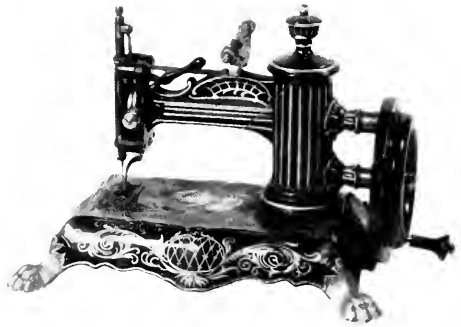
Figure 86.—EMPIRE SEWING MACHINE. Late 1860s. Although an Empire Sewing Machine Co. existed in New York in the 1860s (the predecessor of the Remington-Empire Co.), it is not known whether this machine was manufactured by that same company, which was primarily concerned with producing shuttle machines. This chainstitch machine is marked "Empire Co., Patented April 23, 1863," the date referring again to Ketchum's patent. It is very similar to Folsom's Globe, except that it has claw feet rather than a closed base; the painted designs on the base of both are almost identical to those on the Monitor. Its spool holder, mounted in reverse, is a crude imitation of the Folsom patent. The Empire machines were probably manufactured about the same time as the Wilson machine. (Photo courtesy of The Henry Ford Museum and Greenfield Village, Dearborn, Michigan.)
